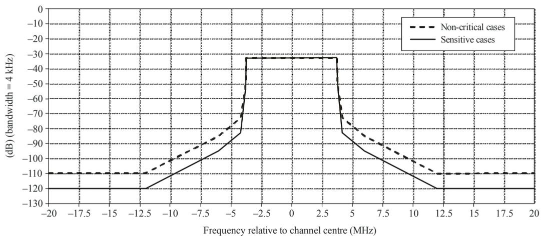
Figure A1-1 Transmission spectrum limit masks for 8 MHz
